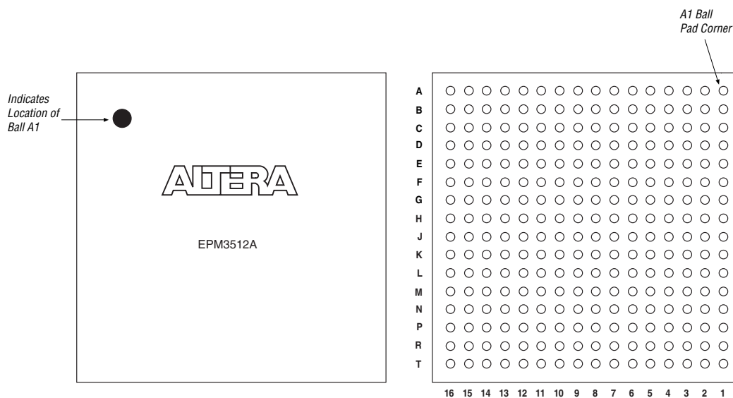
Figure 18. 256-Pin FineLine BGA Package Pin-Out Diagram
