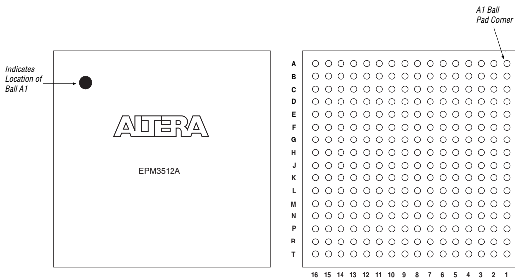
Figure 18. 256-Pin FineLine BGA Package Pin-Out Diagram
