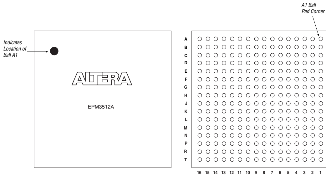
Figure 18. 256-Pin FineLine BGA Package Pin-Out Diagram
