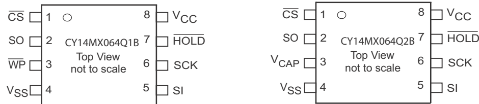
Figure 1. 8-pin SOIC pinout [1, 2]
