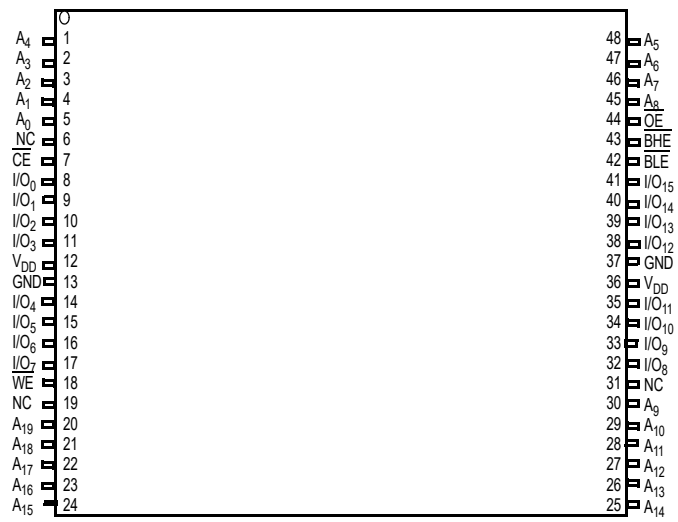
Figure 8. 48-pin TSOP I (12 × 18.4 × 1 mm) Pinout, Single Chip Enable without ERR, CY7C1061G [7] Package/Grade ID: ZXI
