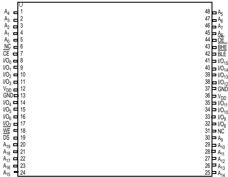
Figure 5. 48-pin TSOP I (12 x 18.4 x 1 mm) Pinout, ERR Output at Pin 6 (Top View)
