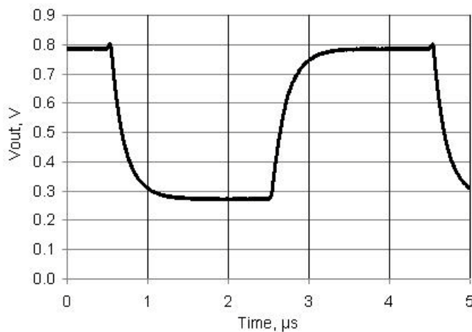
Figure 11-54. VDAC Step Response, Codes 0x40 - 0xC0, 1 V Mode, Fast Mode, V DDA = 5 V
