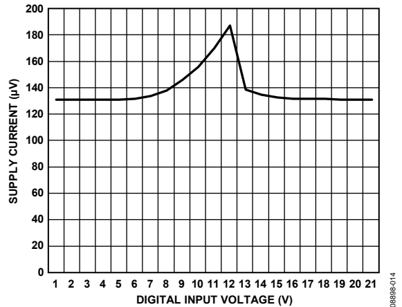
Figure 14. Supply Current vs. Digital Input Voltage
