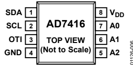
Figure 7. AD7416 Pin Configuration (SOIC/MSOP)
