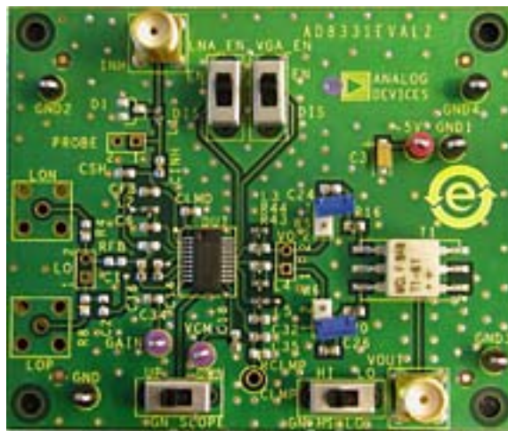
Figure 95. Photograph of AD8331-EVALZ
