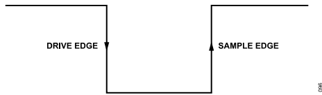
Figure 98. SPI Mode 0 SCLK Edges
