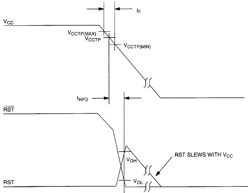
**TIMING DIAGRAM: POWER UP** Figure 8
