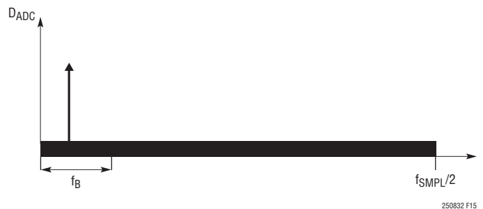
Figure 15. Frequency Spectrum of SAR ADC Core Output
