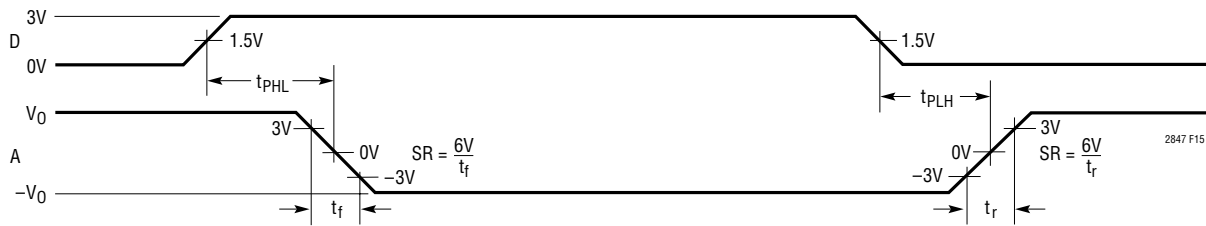
Figure 15. V.28 Driver Propagation Delays
