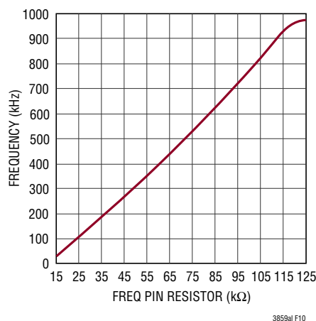
Figure 10. Relationship Between Oscillator Frequency and Resistor Value at the FREQ Pin
