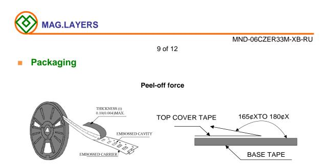
The peel off force of cover tape is 10 to 70 grams in the arrow direction.
