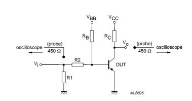
$$\begin{split} V_i = 0.5 \text{ to } 4.2 \text{ V; } T = 500 \text{ } \mu\text{s; } t_p = 10 \text{ } \mu\text{s; } t_r = t_f \leq 3 \text{ ns.} \\ R1 = 56 \text{ } \Omega; \text{ } R2 = 1 \text{ } k\Omega; \text{ } R_B = 1 \text{ } k\Omega; \text{ } R_C = 270 \text{ } \Omega. \end{split}$$
