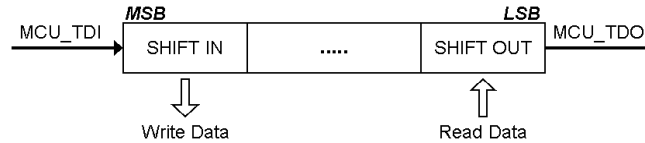
Figure 17-3 JTAG Port Shift Register
