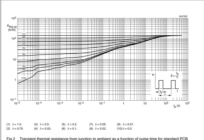
Fig.2 Transient thermal resistance from junction to ambient as a function of pulse time for standard PCB footprint.
