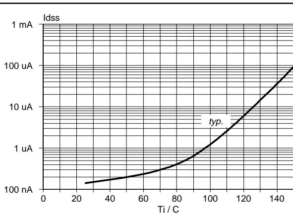
Fig.28. Typical off-state leakage current.
