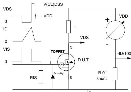
Fig.27. Clamping energy test circuit,  $R_{IS} = 50\text{ }\Omega$ .
