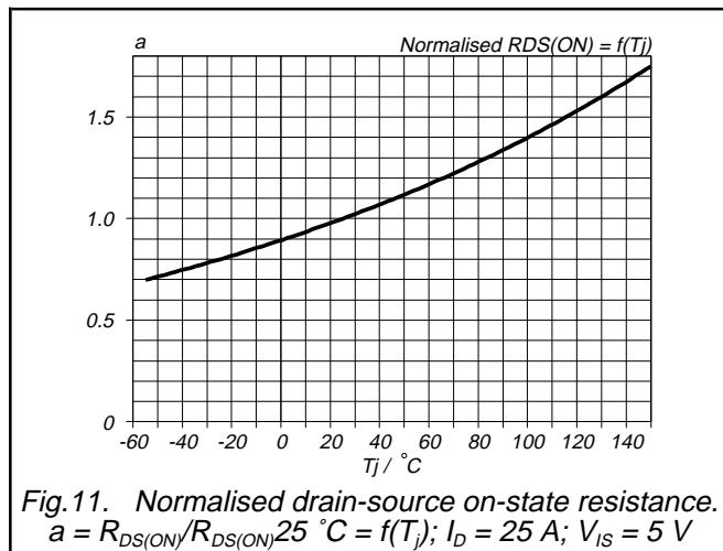
Fig.11. Normalised drain-source on-state resistance.
