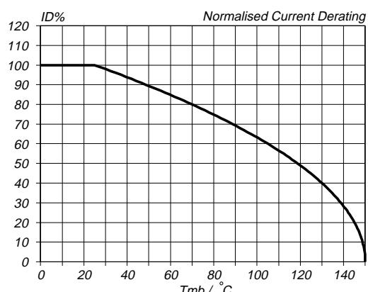
Fig.3. Normalised continuous drain current.
