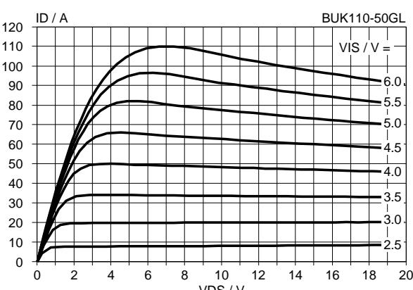
Fig.6. Typical output characteristics,  $T_j = 25^\circ\text{C}$ .
