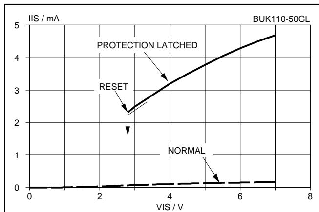
Fig. 18. Typical DC input characteristics,  $T_j = 25$  °C.
