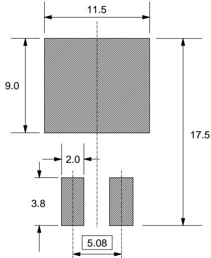
Fig.32. SOT404 : minimum pad sizes for surface mounting.
