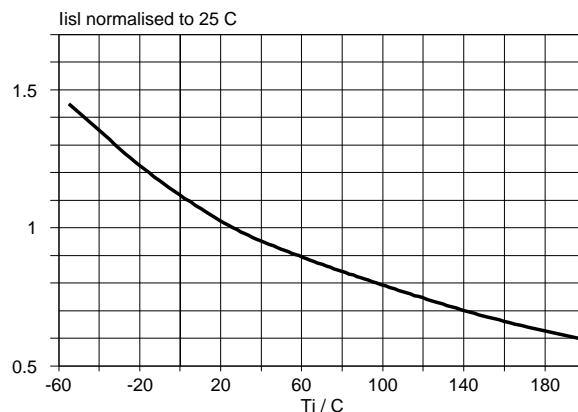
Fig.30. Normalised input current (protection latched).
