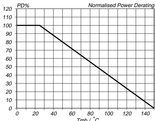
Fig.2. Normalised limiting power dissipation.
