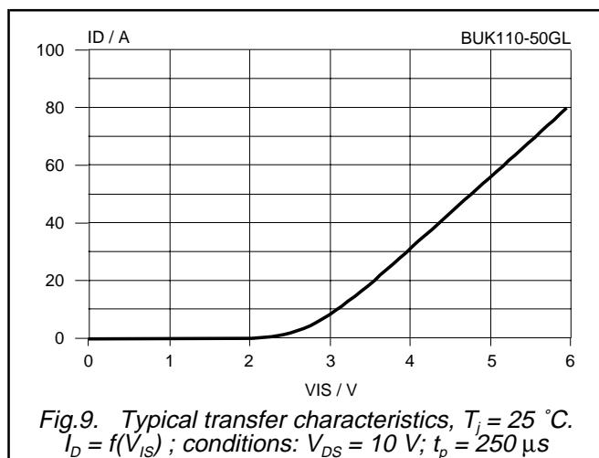
Fig.9. Typical transfer characteristics,  $T_j = 25^\circ\text{C}$ .
