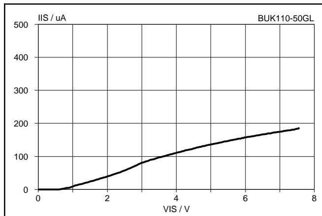
Fig. 17. Typical DC input characteristics,  $T_j = 25$  °C.
