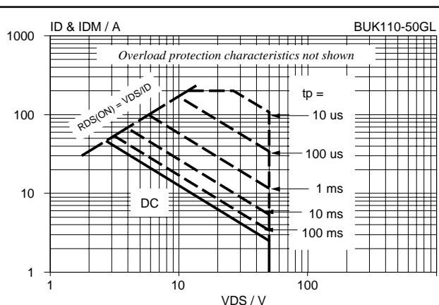
Fig.4. Safe operating area.  $T_{mb} = 25^\circ\text{C}$
