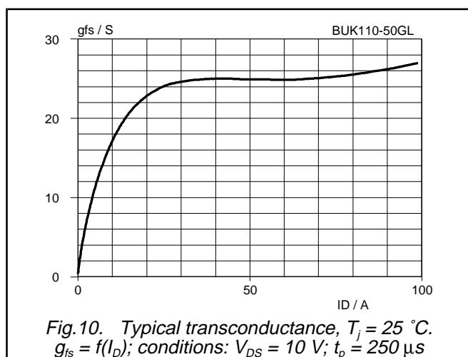
Fig.10. Typical transconductance,  $T_j = 25^\circ\text{C}$ .
