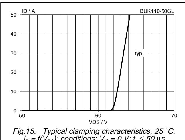
Fig. 15. Typical clamping characteristics, 25 °C.
