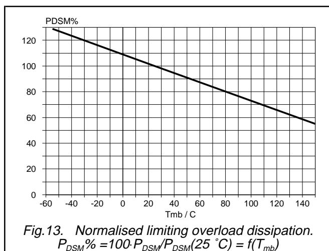
Fig.13. Normalised limiting overload dissipation.
