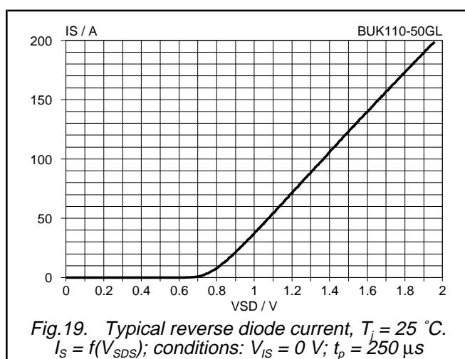
Fig. 19. Typical reverse diode current,  $T_j = 25$  °C.
