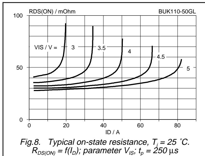
Fig.8. Typical on-state resistance,  $T_j = 25^\circ\text{C}$ .
