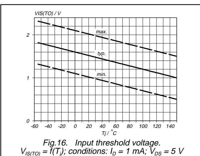
Fig. 16. Input threshold voltage.
