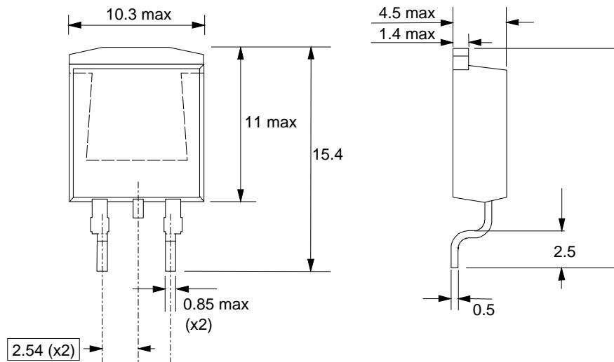
Fig.31. SOT404 : centre pin connected to mounting base.
