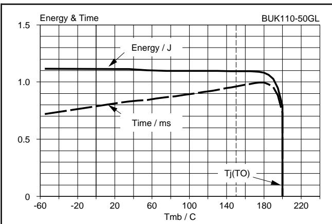
Fig. 14. Typical overload protection characteristics.
