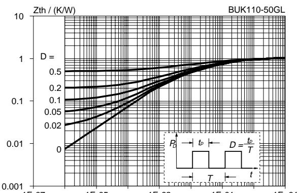
Fig.5. Transient thermal impedance.
