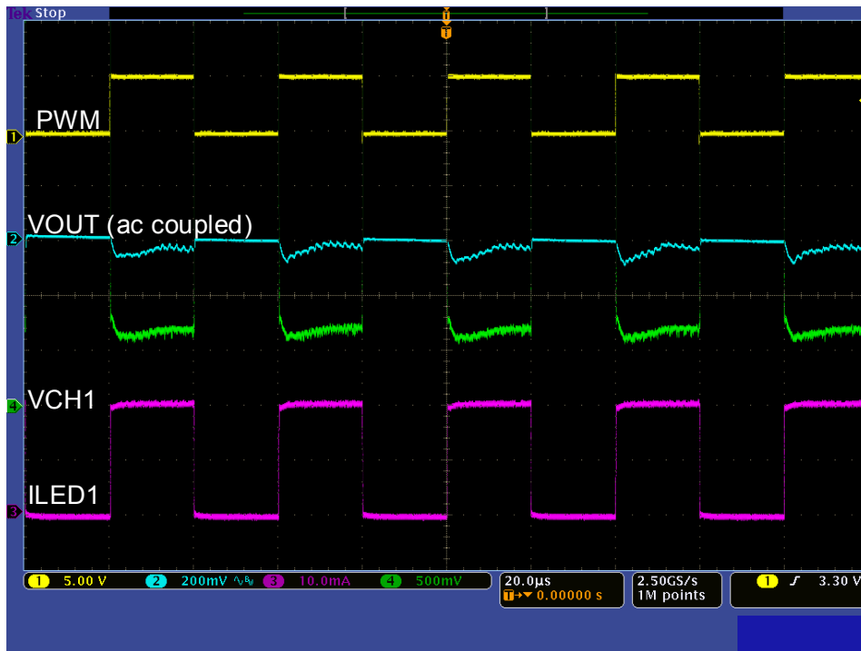
Figure 8. Typical operating waveforms (FPWM = 25 kHz, 50% duty)
