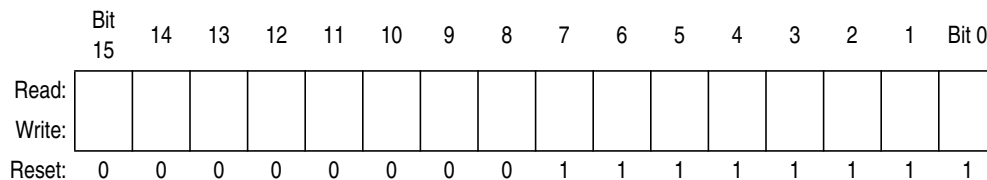
Figure 4-4. Stack Pointer (SP)
