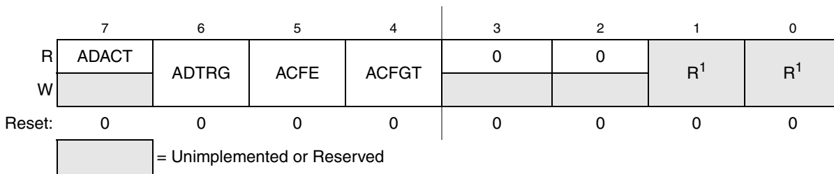
Figure 14-5. Status and Control Register 2 (ADC1SC2)
