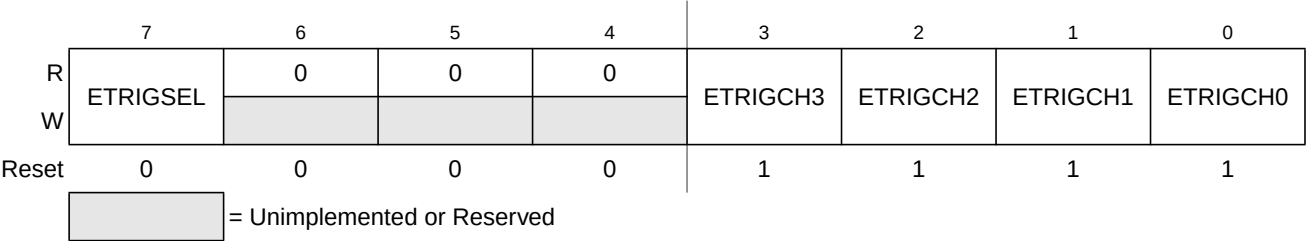
Figure 7-4. ATD Control Register 1 (ATDCTL1)
