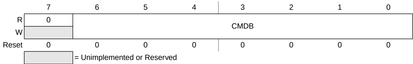
Figure 2-12. Flash Command Register (FCMD - NVM User Mode)
