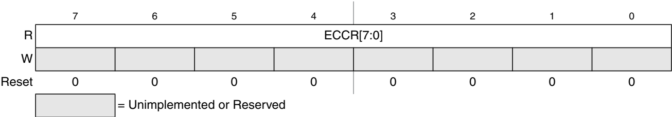
Figure 29-21. Flash ECC Error Results Low Register (FECCRLO)
