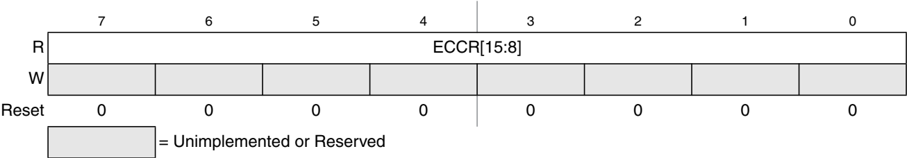
Figure 29-20. Flash ECC Error Results High Register (FECCRHI)
