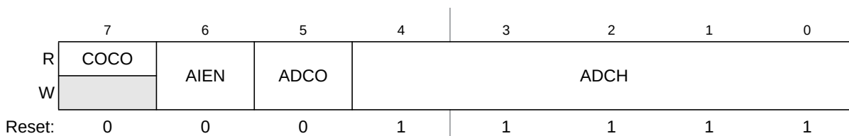
Figure 10-3. Status and Control Register (ADCSC1)
