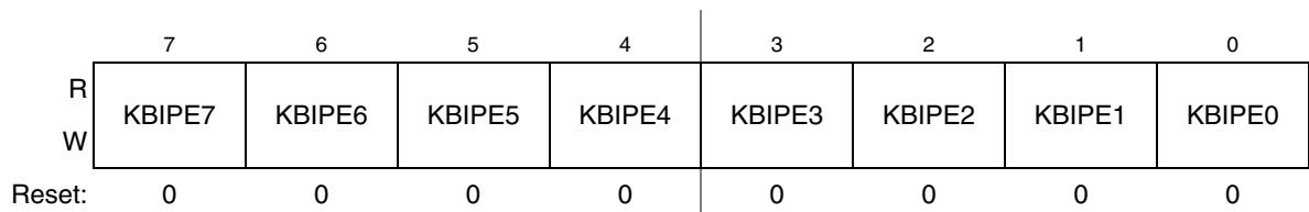
Figure 10-4. KBI Pin Enable Register
