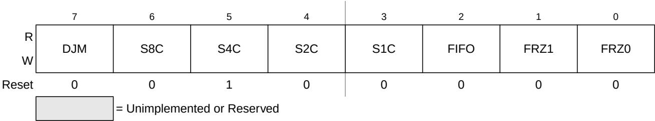
Figure 9-6. ATD Control Register 3 (ATDCTL3)
