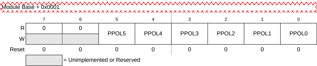
Figure 10-4. PWM Polarity Register (PWMPOL)
