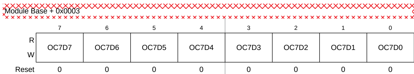
Figure 14-9. Output Compare 7 Data Register (OC7D)
