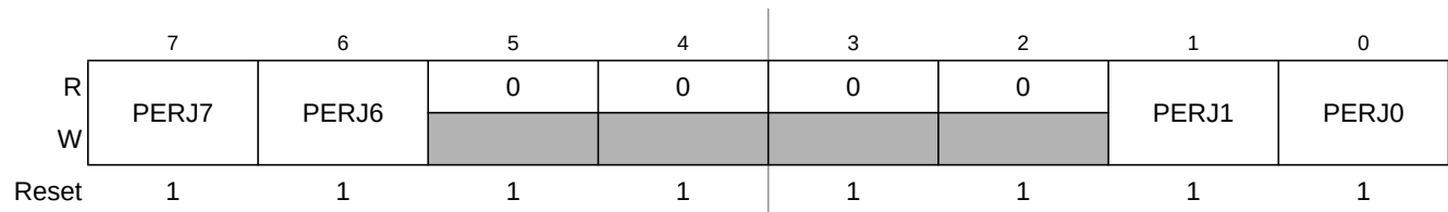
Figure 2-60. Port J Pull Device Enable Register (PERJ)
