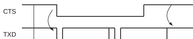
Figure 36-28. Transmitter Behavior when Operating with Hardware Handshaking
