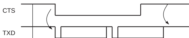
Figure 36-28. Transmitter Behavior when Operating with Hardware Handshaking
