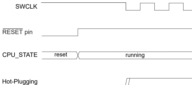
Figure 13-3. Hot-Plugging Detection Timing Diagram
