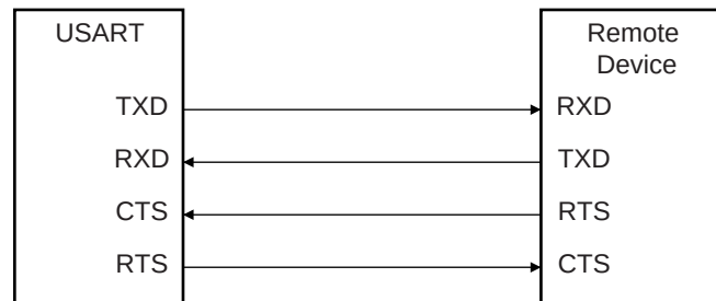
Figure 30-16. Connection with a Remote Device for Hardware Handshaking
