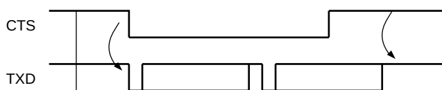
Figure 30-19. Transmitter Behavior when Operating with Hardware Handshaking
