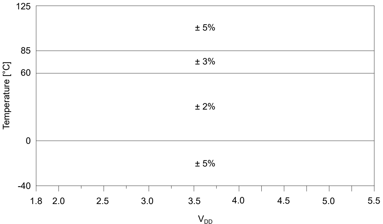
Figure 38-2. Precision Calibrated OSCHF (4 MHz) Frequency Accuracy Over Device V_{DD} and Temperature
