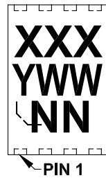
8-Lead DFN (3x3x0.9 mm) (MCP632)
