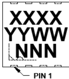
8-Lead DFN (3x3x0.9 mm) (MCP632)
