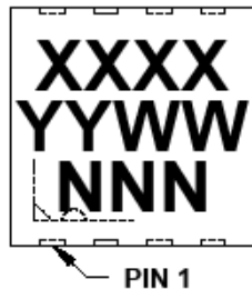
8-Lead DFN (3x3x0.9 mm) (MCP662)
