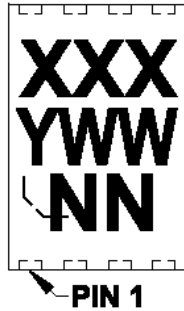
8-Lead TDFN (2x3x0.8 mm) (MCP6V77)
