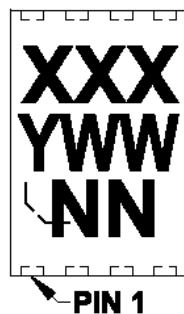
8-Lead TDFN (MCP6V92)
