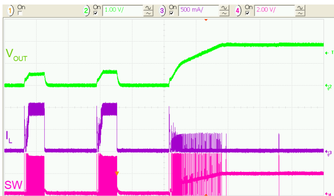
Figure 37. Overload Recovery to Light Load, 50\ \mu\text{s}/\text{div} .
