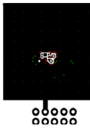
a) 86^\circ\text{C/W} when mounted on a 1 in 2 pad of 2 oz copper
