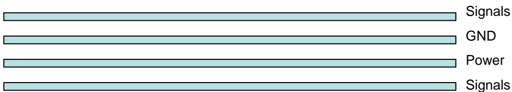
Figure 15: Typical 4-layer PCB construction
