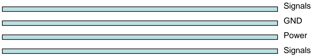
Figure 12: Typical 4-layer PCB construction
