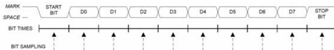
Figure 22.4. UART0 Mode 1 Timing Diagram
