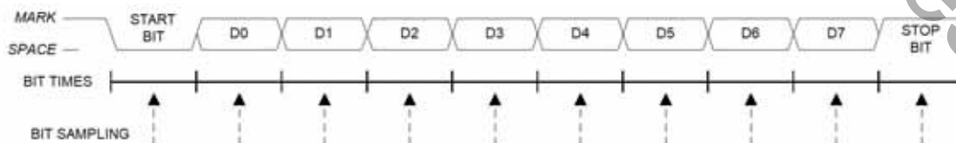
Figure 23.4. 8-Bit UART Timing Diagram
