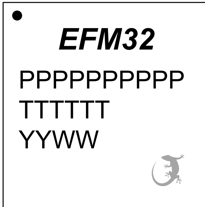
Figure 10.3. TQFP100 Package Marking
