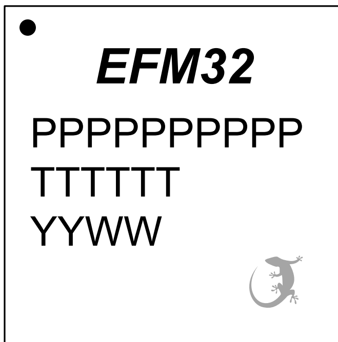
Figure 10.3. TQFP100 Package Marking
