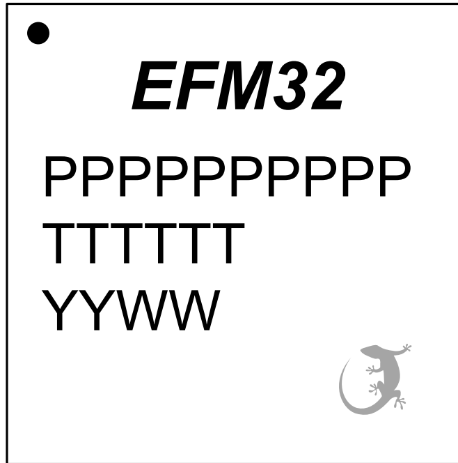
Figure 9.3. BGA112 Package Marking
