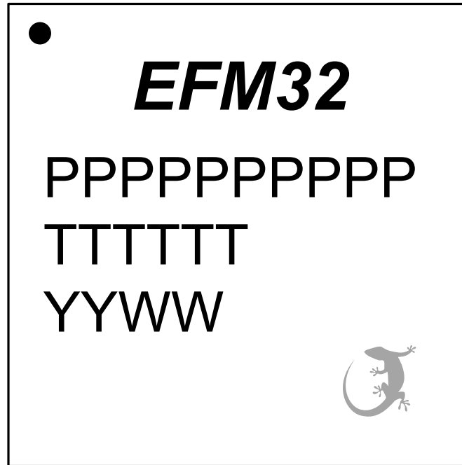
Figure 7.3. BGA112 Package Marking
