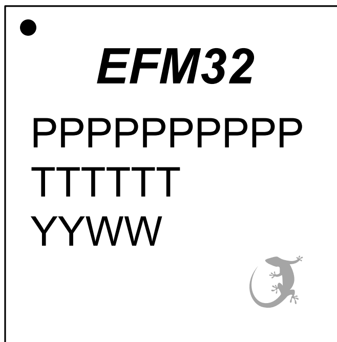
Figure 8.3. TQFP64 Package Marking
