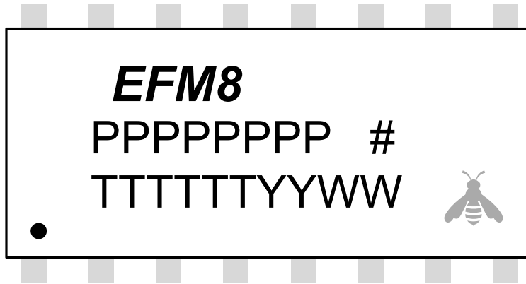
Figure 9.3. SOIC16 Package Marking
